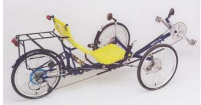
Here are some pictures of the rear suspension GTO-E model. Note this is our latest GTO-E model with the new Ergo seats, and anti brake steer steering. Unlike some RS systems, the luggage is also suspended. Other options on this trike are the disc brakes, lightweight wheels, and 12 volt B&M lighting system.
