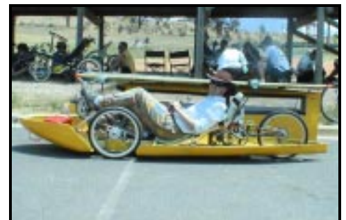
Chris Curtis and his solar assist trike Sun-strike. The top half of the fairing with the solar cells can be seen behind Chris.
