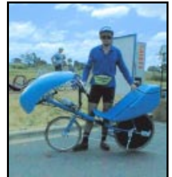
Peter Heal (8) had spent a busy year making modifications to his recumbent bike. New this year was above seat steering, rear wheel disk and the front and rear fairings
