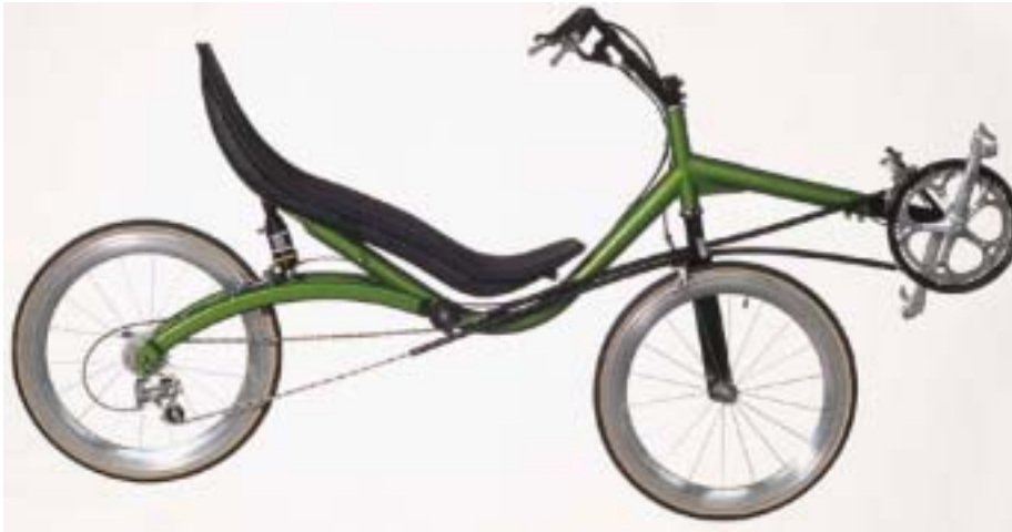
Shockproof with 'monoblade' suspension fork, 451mm aero wheels, and no rack fitted.
