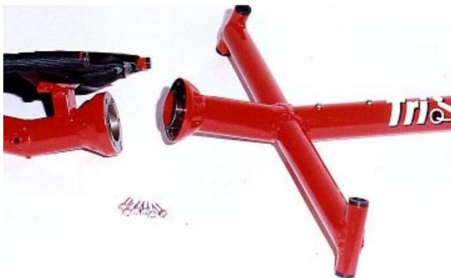
I decided that a single break in the middle would be the ideal compromise between compact size and simplicity of fold. That sounds easy enough, just put an S&S in the middle right?... Well no. Upon some research into the S&S coupling I discovered it has one (very) limiting factor. It cannot be placed in middle of a cantilevered member and is intended for triangulated applications (such as a diamond frame).
