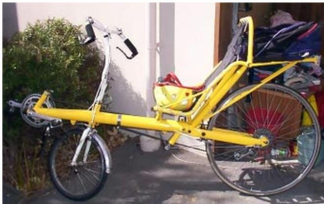
Bruce has a very nice aluminium trike that he designed and had (I believe) Gavin do much of the fabrication of. It's based on the suspended Trice Micro, with Windcheetah style ASS. It felt light, and Bruce says 16kg in race trim. Riding it was interesting - the suspension makes it almost plush to ride, and the mechanical discs certainly make it stop quickly. But it's twitchy like a Windcheetah and the suspension does tend to squat a bit under
