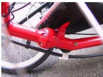
When I was testing the prototype frame, I rode it around for a few hours with the bolts only done up hand tight and also with the tension side bolts missing without any problems. Although this relieved some early fears I had had, I would not recommend trying this during every day use.
