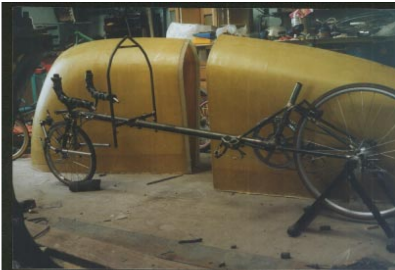
Completed kevlar copy sits behind bike, unpainted and windowless.
