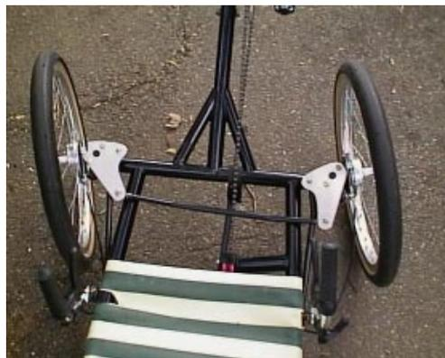
The included angle is 11 degrees, the same as that of the steering tube on the cross-member, so the axles are dead horizontal. At the top of each kingpin is a bell crank.
