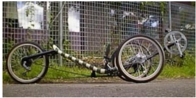
The frame is made up of two long bent bits. Each has two bends, and they are not in the same plane, so it may be a little tricky to visualize. On the next page is the plan you take to the exhaust bender.
