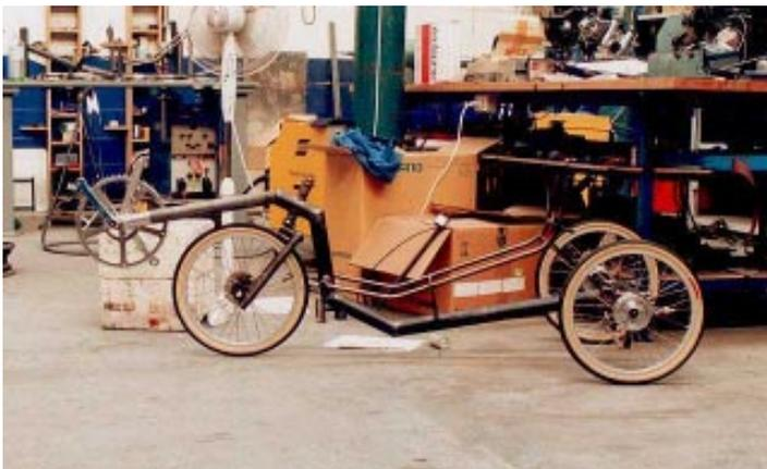
but three wheels or more are allowed to compete. The rules state that the machine must have three or more load bearing wheels and that tilt steering has proven insufficient in the past and designs of that nature need to be preapproved before they can compete. So I set about making a trike that could lean into corners, the security of a trike, but the corner speed of a bike.
