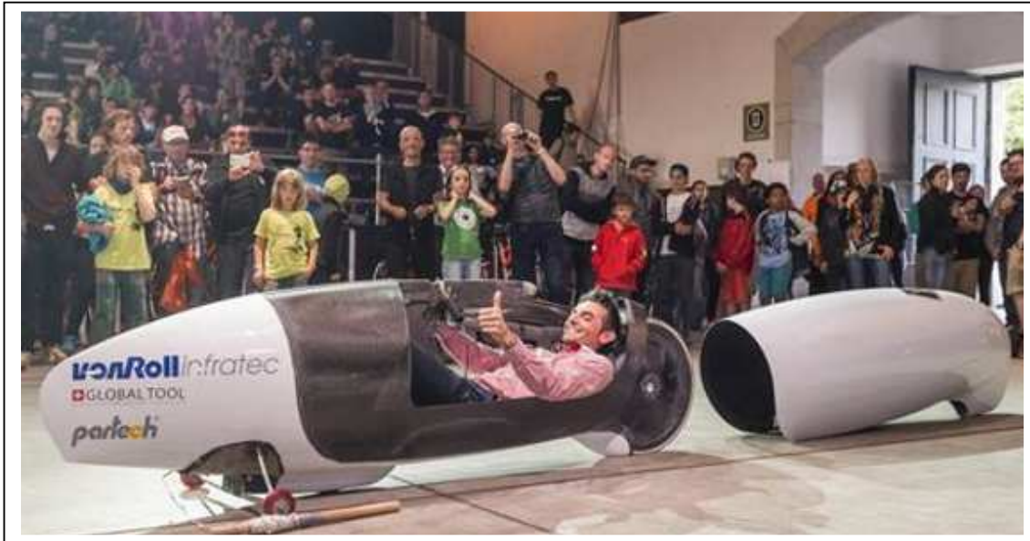
Metastretto with front fairing removed and trolley used for support when starting.
