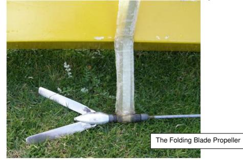
Rick is now working on V15 (yes that's version 15) of his pedal powered boats and says his sister wants a boat like his so he is working on an integrated hull design for her with a target weight of 15kg. It's Pink too. Note there is no chain – just a direct drive gear box to the propeller shaft.
