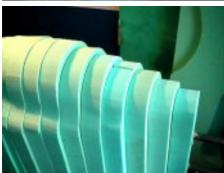
First Cad drawing was made of the proposed shape. This was translated onto polyurethane foam sheet and bonded together on a steel datum frame. Just imagine taking to the final shape with a giant bread slicer and then gluing it back together....
