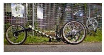
The frame is made up of two long bent bits. Each has two bends, and they are not in the same plane, so it may be a little tricky to visualize. On the next page is the plan you take to the
