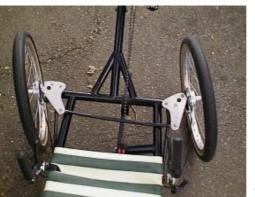
The included angle is 11 degrees, the same as that of the steering tube on the crossmember, so the axles are dead horizontal. At the top of each kingpin is a bell crank.
