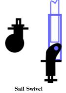
fits over or in the spar tube for a socket. Remove the wheel, then push the tube into the wheel mount, drill it and fix it in position with the bolt that held the wheel. Use another self tapper or two into the bottom of the tube to stop it tilting back. I thought the bolt would hold it, but the wind pressure soon dragged the socket back. It needs quite strong fixing, there's a lot of leverage.
