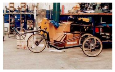
but three wheels or more are allowed to compete. The rules state that the machine must have three or more load bearing wheels and that tilt steering has proven insufficient in the past and designs of that nature need to be preapproved before they can compete. So I set about making a trike that could lean into corners, the security of a trike, but the corner speed of a bike.
